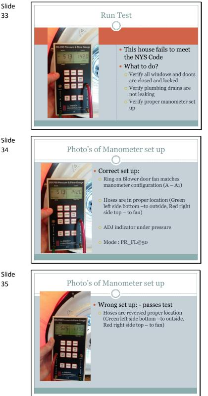
Run Test (since wind pressure is constantly changing the pressure will jump from -45.0 Pa to -55.0 Pa or more)
