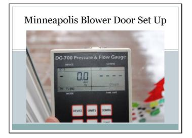
Adjusted Pressure is 0 Select appropriate Device (Blower Door 3 is standard, Blower Door 4 is a 220V version, Duct Blaster Fans can be used as well) Select appropriate Configuraton (Ring size)
