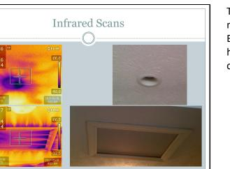
Top Photo Set – Recessed light not sealed Bottom Photo Set – This attic hatch has a gasket. Caulk trim to ceiling, add weight to the hatch
