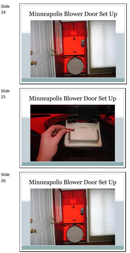
Manometer board installed onto frame (optional)
