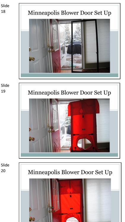
Assemble Frame, rough size frame into door opening, outdoor pressure hose is placed away from fan (around a corner)
