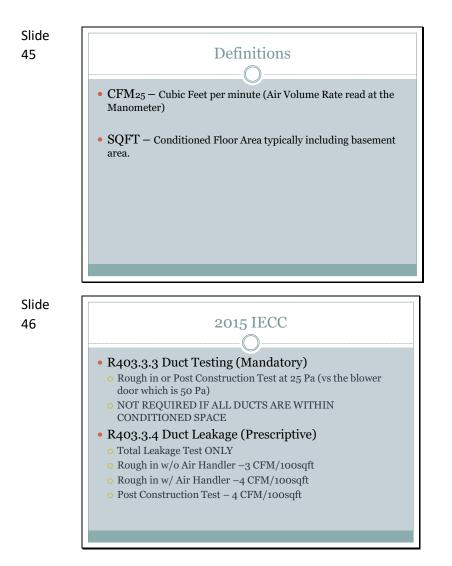
CFM25 – Duct Leakage Test Result SQFT – conditioned area of house, typically includes the basement but excludes any floor area with walls less than 5' tall (ie: Next to a knee wall)
