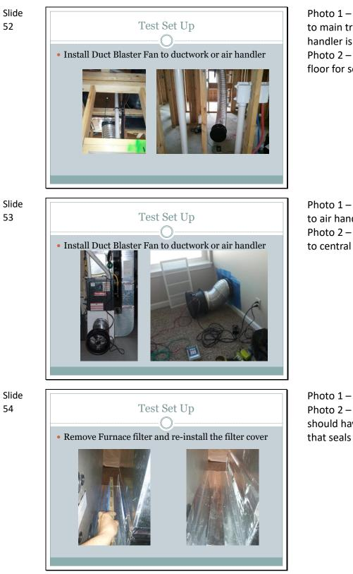
Photo 1 – Duct blaster connected to main trunk line before the air handler is installed Photo 2 – Duct blaster fan on the floor for set up
