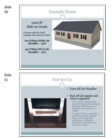
Run through an example house – This is a slab on grade version – if it had a basement it probably wouldn't need a test
