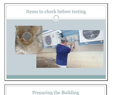
Photo 1 – Floor Drain – may be dried out, fill before test Photo 2 – Continuously operating HRV/ERV supply and exhaust
