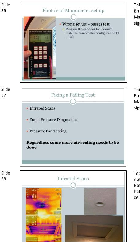
Things to watch out for: Operator Error – Incorrect configuration on Manometer – changes results significantly
