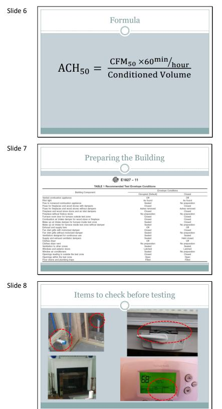
Put house in wintertime conditions. Only thing you are allowed to completely seal off is an HRV/ERV system supply and exhaust.
